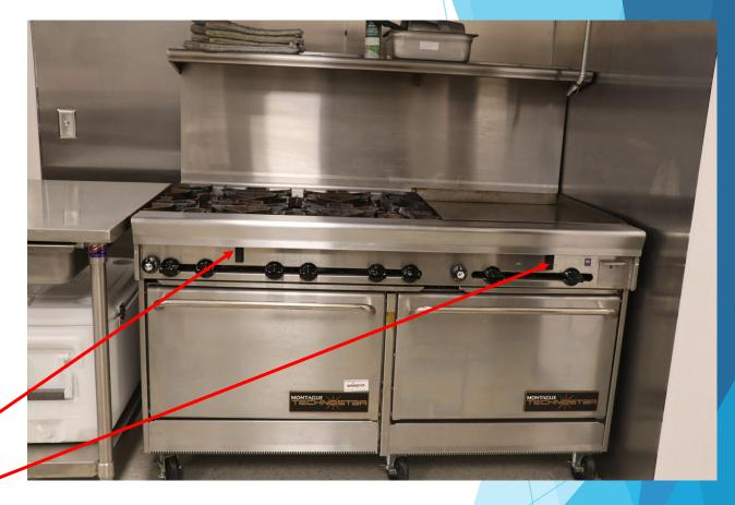
Set oven temperature 50 degrees lower when using the commercial convection ovens. i.g. if the recipe calls for 350 degrees F set the oven temperature at 300 degrees in the convection oven. Make sure the blower toggle switch is in the Up Top On position when baking.
