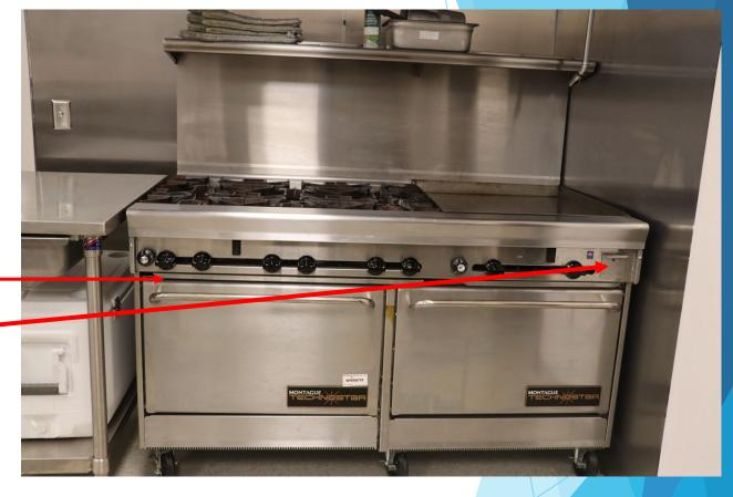
Empty the griddle grease tray of any grease and soapy water remaining. Remove grease tray, wash, dry and return to the range'
